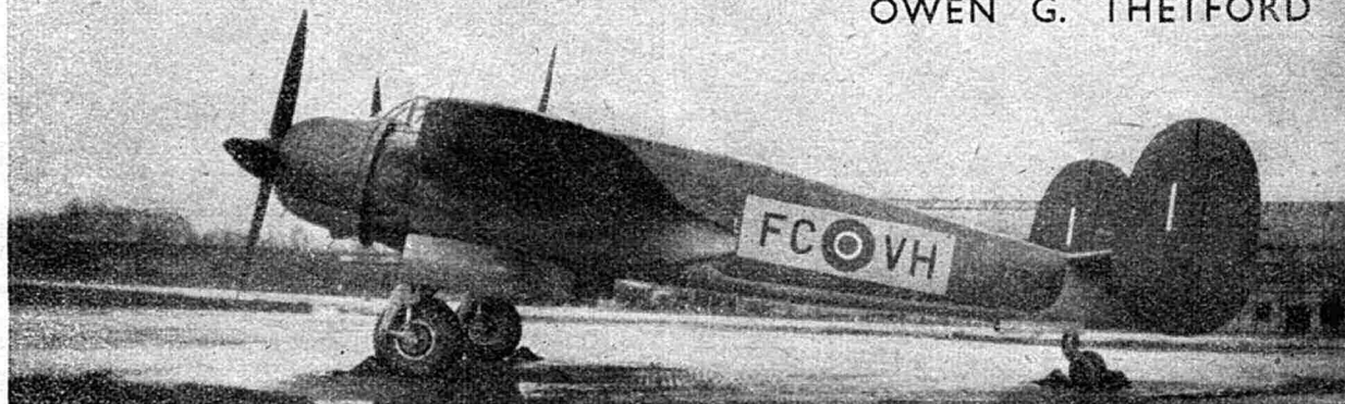
Photo: G. A. Cull. MODERN TRAINING : First picture to be published showing the Bristol Buckmaster fast conversion trainer in service with Flying Training Command. Only a limited number of Buckmasters was built and production ceased some time ago. Of special interest is the yellow panel on the fuselage, against which the code letters are painted.
