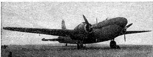
Photo: Yickers. HIGH FLYER : A rarely photographed Wellington—the Mark V high-altitude version with the pressurised cabin. This hitherto unpublished view was taken early in 1941.
