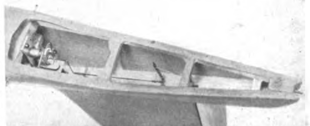
Left is the Aeromodeller version with magnetic actuator installation and a similar view of Walt Good's prototype with rubber-driven actuator.
