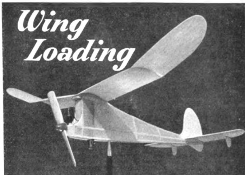
2½ ozs. per sq. ft. This campus powered midget was designed with the aid of the information given in this article.
