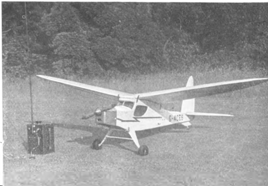
The author's semi-scale radio model of large size, powered with an American Forster 14 c.c. petrol engine. Petrol engines need not be elaborately screened to prevent interference if simple remedies are adopted.
