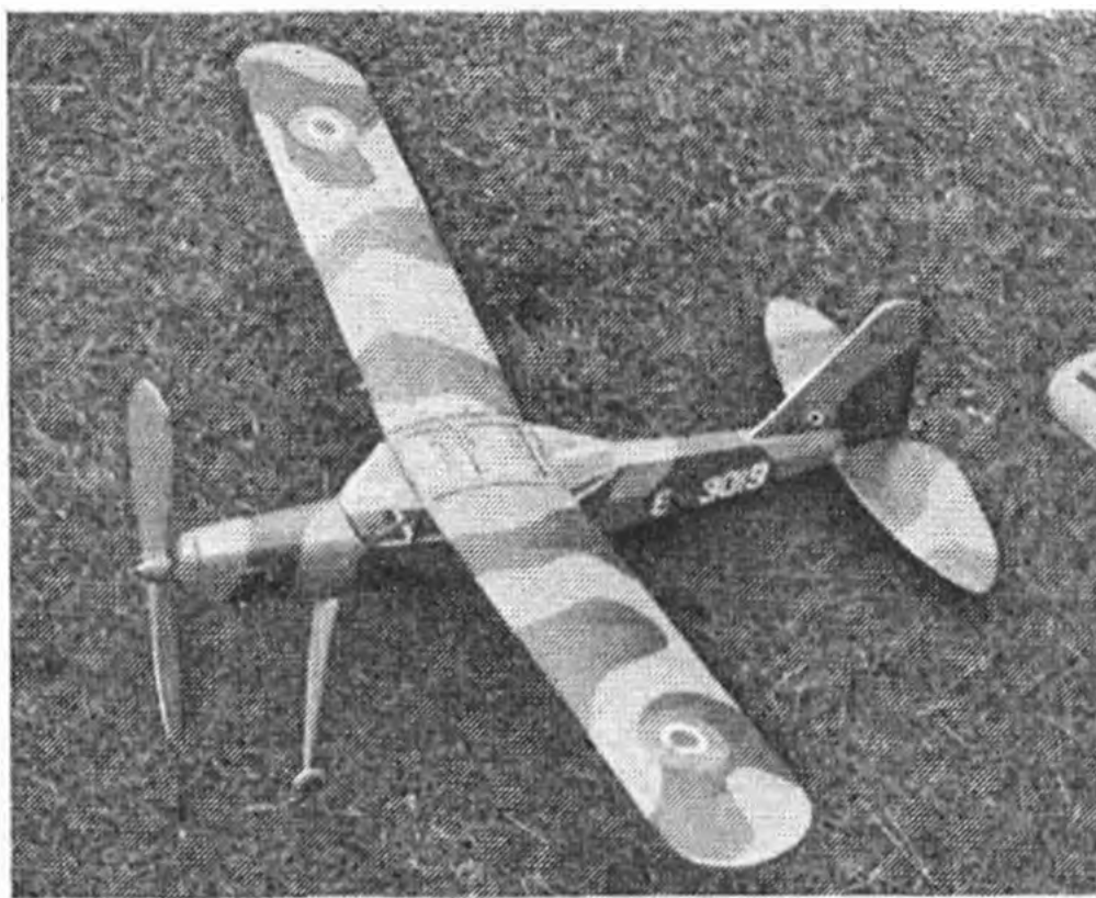
Two views of this attractive semi-scale Army Observation Post 'plane reveal simplicity in structure coupled with commendable realism. Model is sturdy enough for all-weather flying, yet capable of consistent flights of more than a minute.
