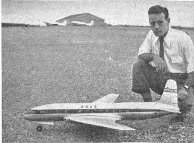
Scaled up from an A.P.S. scale drawing, this 2-in.-1-ft. De Havilland Comet in jet powered. John Stivala of C. Paula in Malta is the ambitious constructor, and in the inset photo the Swiss Furrer jet is seen installed in the starboard outer nacelle. Another similar jet will be fitted to the port wing before flight trials. Note the flap to aid lift and improve landings.
