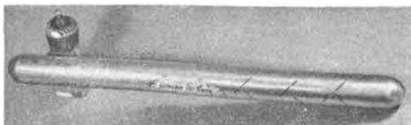
Mar-Lee Silencer dwarfs an Ohlson 29; reduces exhaust noise to "Barbini" level, revealing piston slap and big end knocking
