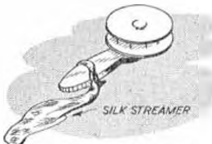
Large silk streamer tied to glider which prevents loss in long grass.
