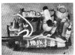
Inside the latest E.B. Transistrol receiver, showing compact arrangement of components within 2 1/2 x 1 1/2 in.
