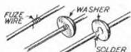
Fuse wire binding strengthens soldered joints, e.g. washer on propeller shaft, etc.
