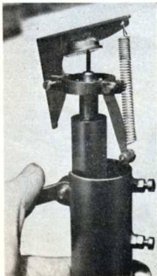
At left, Cambridge Club pylon head. Thumb pressure on the actuating trigger (normally pulled down by a cable from the joystick base) is seen to push the control arm upwards, in effect this attitude gives down elevator. The two screws on the main pylon vertical tube are used solely to locate pylon head securely. Heavy weights are necessary on the base
