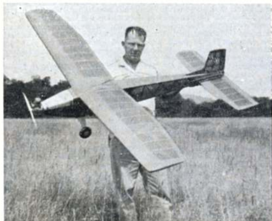
Peter Grunbaum of AUSTRIA designed the 60 in. taper-wing stunter with short span flaps, radial cowl round the O.S. Max 35 and super finish. Right: Stunt Champ. Gabris' design, and below Henry Struck's Met-model.
