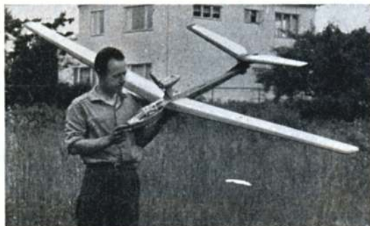
A Friberg of Tyringe, SWEDEN made this power assisted glider for r/c with a Webra Record 1.5 in the pylon. Span is about 100 in. From SPAIN, the scale c/l Sparrowhawk for an E.D.246 Racer is by Alberto Dalmau of Barcelona.
