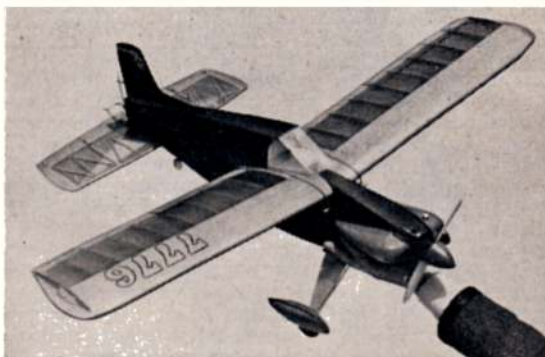
Ron Moulton's "Loopy Lou" test model for 1 c.c. and moulded acetate "bath" to protect Rx, below
