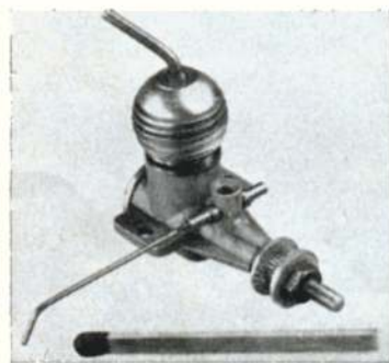
Left: The diminutive 0.25 c.c. Hungarian engine compared with a standard match. Right: the E.D. Racer with throttle and the Webra 3.5 Bully carrying effective silencer, throttle and vacuum pump.
