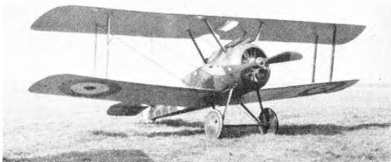
Right: The Bristol Scout was the first British aircraft to go to France fitted with a machine-gun interrupter gear; only a few machines were equipped in this way, and photographs of them are rare. This Scout D's Vickers gun was synchronised by the Vickers-Challenger interrupter gear, the link rod of which can be clearly seen. The fact that the gun had a chute for empty cases, indicates that a disintegrating-link type of ammunition belt was in use when this photograph was taken.
