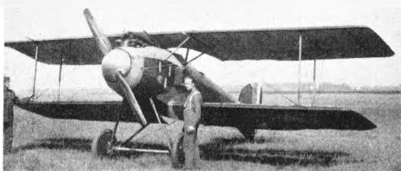
Above heading: This captured Halberstadt DIII has also acquired a British pressure head. Its British markings have been applied with great care and in accordance with prevailing British practice. The small lettering at the top of the white stripe on the rudder reads:— A.R.S.F. 4541 19 6 17
