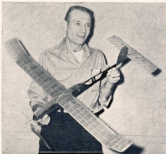
Lyle Elyea of Illinois who has done much to promote the Coupe d'Hiver rubber model class in the U.S.A. with his model which gained 3rd individual placing in the March '63 postal international. Note change of fuselage section to triangular aft of the motor peg.
