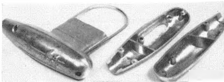
Above shows both assembled and disassembled Merco silencer. Note the two half baffles and offset exhaust inlet to give a swirling effect to the exhaust gases.
