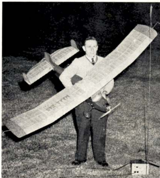
The author holds aloft his "Lucky Star", 7 ft. 2 in. wingspan O/D model. As well as being a night flier "Lucky Star" also carries a camera for daylight photography. Radio operates rudder, motor, elevator or camera from single channel cascaded escapements.
