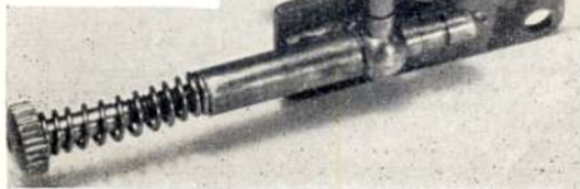
Fox 29X-BB needle-valve assembly is soldered to a steel plate which also serves as a means of retaining and adjusting the valve rotor.
