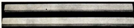
Spruce and Obechi grain differ as shown by strong grain spruce strip at the top and very slight grain in Obechi below.
