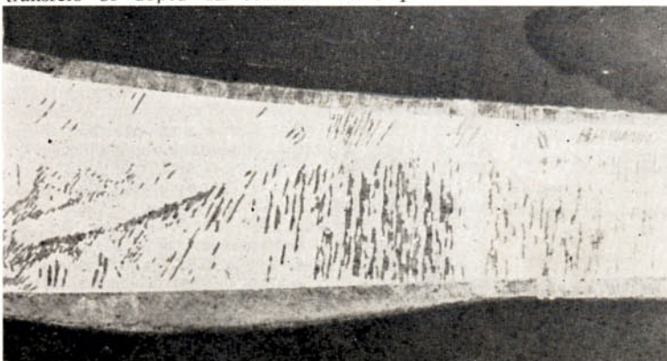
Close up view of two mistakes in finishing. Masking tape covering the white strip has been removed quickly at 90 degrees to the work and not doubled back on itself to reduce surface tension, hence the tissue shows through, where painting is pulled off. Butyrate Aerosol dope was applied over Nitrate clear dope and did not bond, thus it retracted from the white edge line as the second error.
