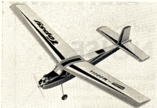
Ever popular Graupner "Topsy" Kit design, ideal for a wide range of engines and equipment. Needs a spot of centre section strengthening for rough field work.
