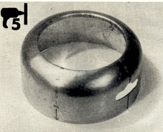
Polish all the hammer marks off with a fine buffing wheel or by hand with emery cloth, then trim all edges including the join seam.
