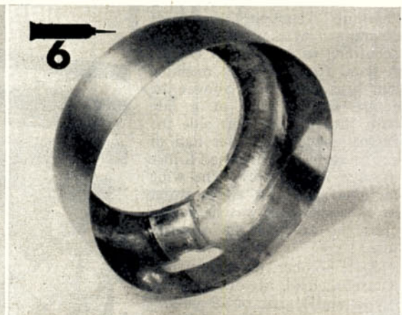
Finish the seam off with a patch of aluminium Araldited to the inside, then give it a final polish and it's ready for the model.
