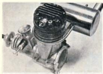
Left, the 1970 Fox 59 fitted with Irvine silencer. Note the characteristic position of glow plug for this engine—lying almost horizontal to the head, on the transfer side.
