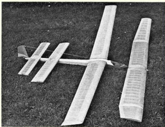
Alternate wing surfaces on Trevor's model permits an immediate, and accurate, comparison of flight characteristics. Larger wing has flat-bottomed wing section for higher airspeed.
