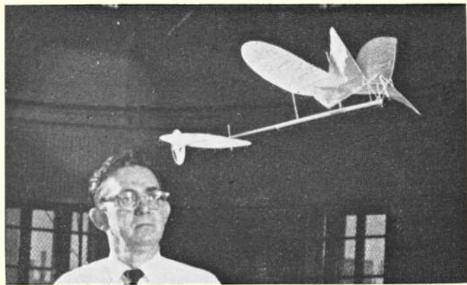
The designer has plenty of opportunity to watch the flight characteristics of his ultra-lightweight birds as the forward velocity is very low. Sudden movement of a person standing this close could seriously affect the flight!
