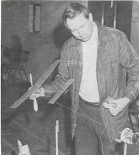
Better known, perhaps, for his exploits with R/C scooters and motor-cycles, Blackburn's John Bridge turned his hand to Easy B at the Southport meeting. Note balsa stiffening employed on fuselage, plus use of electrically powered winder/counter/torque motor – also seen above.
