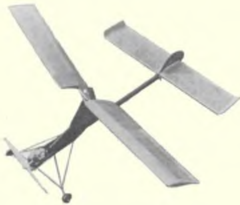
Model No. 1 featured a rotor diameter of 36in. and weighed a total of 18oz. which included ballast. Power was provided by a Mills .75cc. Drawing at right is to 1/12th scale.
