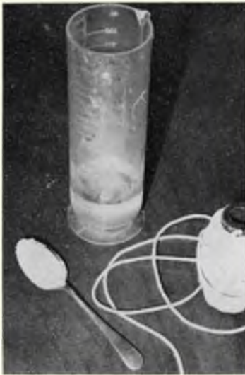
A photographic measuring cylinder, a ball of suitable string, a quantity of saltpetre, and you can go flying safely once more with 'home-grown' dethermaliser fuse - and a reliable D/T action too!
