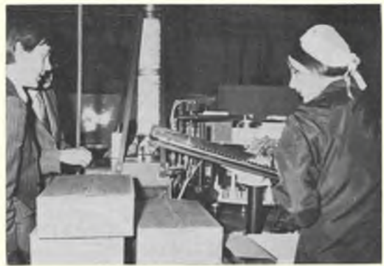
Above: tubes of adhesive are filled, the ends crimped up, and then continue the journey along the many feet of conveyor belt. Below: each and every can of epoxy paint is check-weighted against a standard.
