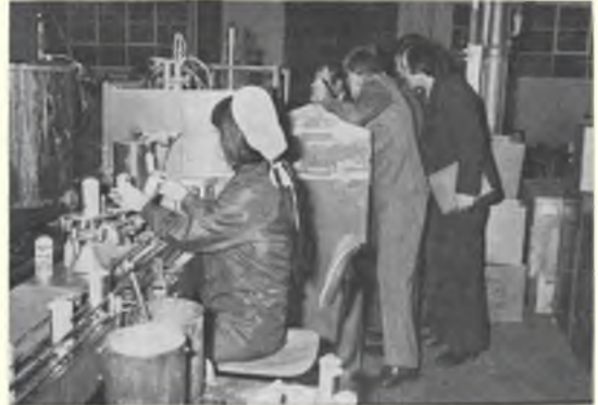
Above: tubes of adhesive are filled, the ends crimped up, and then continue the journey along the many feet of conveyor belt. Below: each and every can of epoxy paint is check-weighted against a standard.
