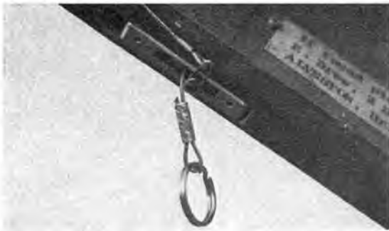
View on underside of fuselage showing Maxaid CTU in slot - also the wire trigger extension for timer connections. Unit weighs just 8 grammes and measures 30mm x 30mm x 5mm.
