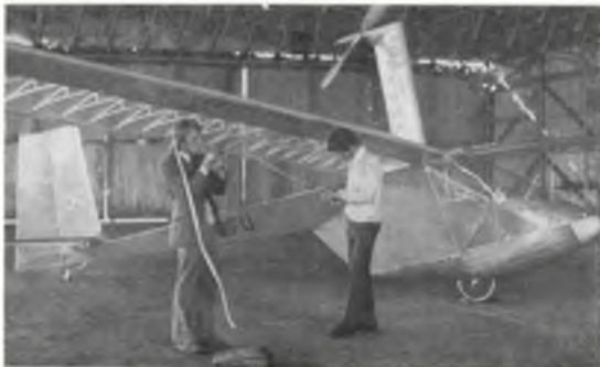
Roger Hardy at work on Dragonfly at Prestwick. This machine is now taken over by Ron Frost and has required modification to overcome its reluctance to rotate nose-up for take-off
