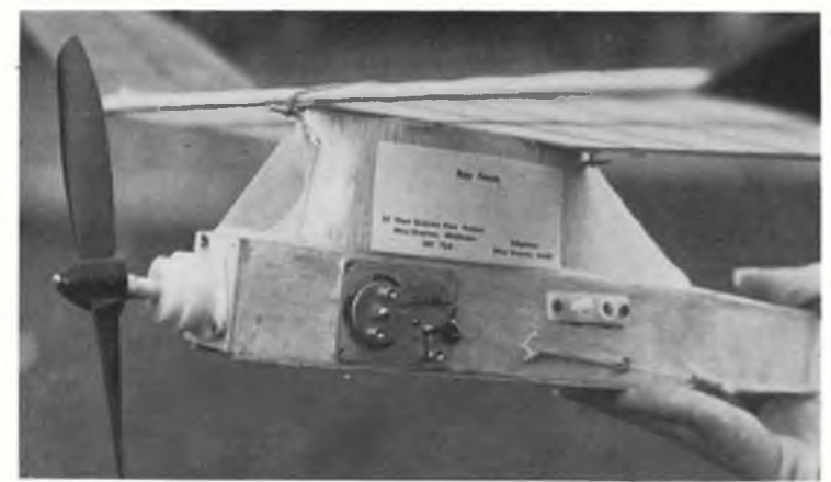
Two views of the VL101 system installed in the Electro-Lite. Note the very simple mounting method used – the motor is simply screwed to a ply former which has a circular hole cut in it to accept the rear of the motor case. Fitting of the clockwork dethermaliser proved to be a very worthwhile precaution.
