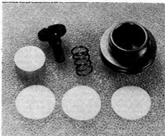
Parts of the DDD Cox 049/051 size diesel conversion kit showing (clockwise from head) three fluorocarbon seals aluminum contra-piston compression screw and spring.
