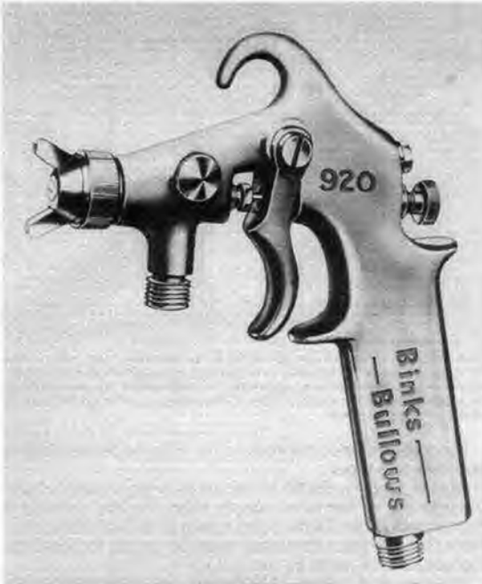
The Binks Bullows 920 unit typifies the style of the hand-held spray gun. Lower connection (at base of handle) is for air supply pipe, and screw connection in front of trigger is for paint supply.
