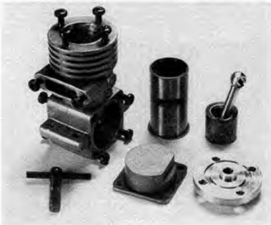
Parts of the Kingcat 1.49. Design and construction is somewhat different from traditional small diesel practice.
