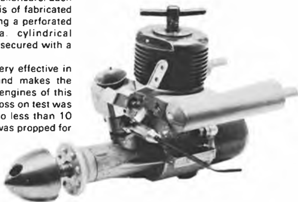
M.E. Snipe R/C with silencers fitted.
