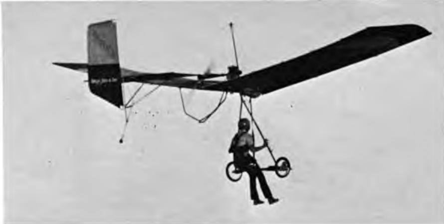
Left: the P-Fledge is one powered variant of the famous hang glider. Only seven wing ribs hold the aerofoil! Above: Quicksilver 2-wheeler prepares for foot assisted landing at all of 15mph ground speed. Note extended tailwheel.
