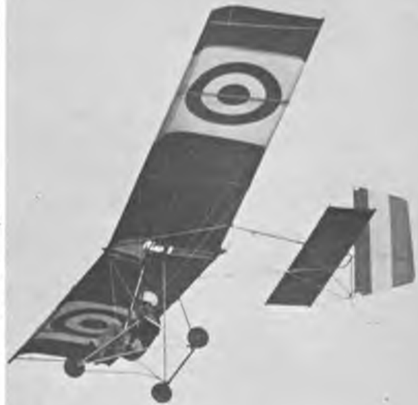
Most popular is the Eipper Quicksilver, this one with French roundels. Engine is a pusher, mounted above wing with prop at trailing edge.
