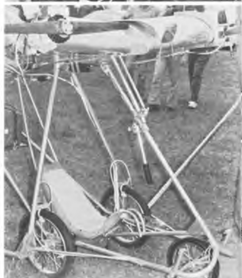
Above: 'Doublequick' twin engine arrangement by Eipper and right: the Lazair with the 100cc engines on leading edge, pendant control column - even brakes on the wheels.
