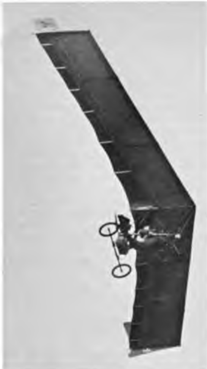
Left: the P-Fledge is one powered variant of the famous hang glider. Only seven wing ribs hold the aerofoil! Above: Quicksilver 2-wheeler prepares for foot assisted landing at all of 15mph ground speed. Note extended tailwheel.
