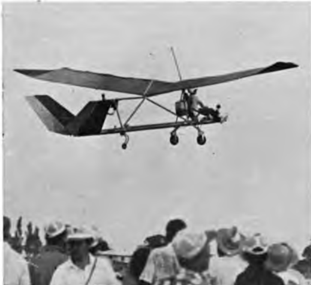
Left: the Hummer combines ruddervators on Vee tail, with generous dihedral. Engine is mid-mounted as a pusher with pilot unusually forward. Below: manoeuvrability of the P-Fledge on approach, using pilot seat shift and tip rudders makes microflying look deceptively easy.
