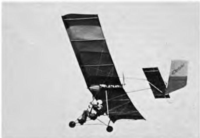
Left: the P-Fledge is one powered variant of the famous hang glider. Only seven wing ribs hold the aerofoil! Above: Quicksilver 2-wheeler prepares for foot assisted landing at all of 15mph ground speed. Note extended tailwheel.
