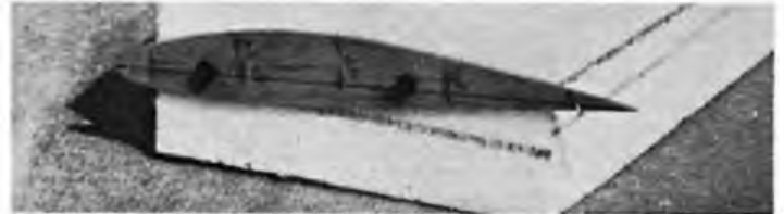
Tilting the tip template at an angle to the centre line to give washout
