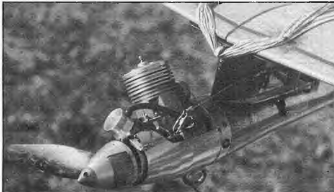
Above: long awaited new Rossi 15, distinguished by black anodised head, failed to live up to expectations. Trumpet air intake on Anton Webber's motor claimed to boost power by 500rpm. Right: single blade prop gives higher efficiency with less drag on glide than two blader as used by Saukenon, Finland - new folding props may be even better!
