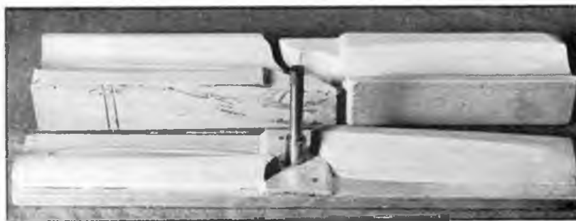
Metal experimental TR prop originally mounted on conical hub turned from plywood. Below mould for a Larsson prop. This mould illustrates built up centre for cuffed root, double diameter centre rod and engraved identification on rear hub.
