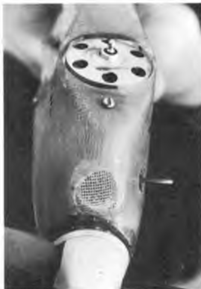
Above: neat tow line load tester used by European Championships organisers at Zulpich. 2kg weight rests on micro switch in circuit of battery-powered bicycle hooter. When tow line load reaches 2kg hooter sounds. Left: Ray Monks' F1C cowling uses a piece of nylon mesh moulded into the fibreglass to keep dirt out of the Rossi air intake.
