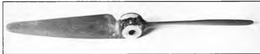
Below TR prop with hub faces trued with copper discs
