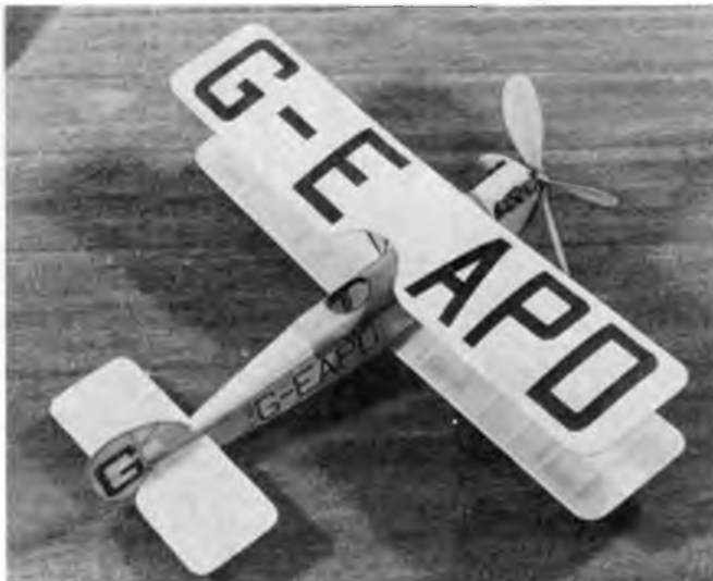
Left: author's Boulton and Paul P9 is 18" in span for rubber power using very light weight construction in conventional materials. Above: this Ansaldo SVA5 was built by Mike Hall of Walsall for CO 2 power. Features sheet balsa fuselage and Xerox paper covered flying surfaces.
