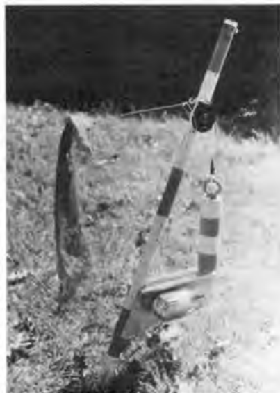
Above: neat tow line load tester used by European Championships organisers at Zulpich. 2kg weight rests on micro switch in circuit of battery-powered bicycle hooter. When tow line load reaches 2kg hooter sounds. Left: Ray Monks' F1C cowling uses a piece of nylon mesh moulded into the fibreglass to keep dirt out of the Rossi air intake.
