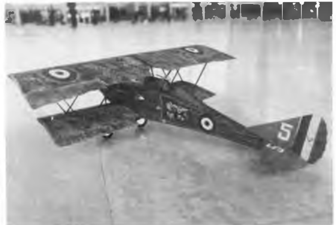
Left: author's Boulton and Paul P9 is 18" in span for rubber power using very light weight construction in conventional materials. Above: this Ansaldo SVA5 was built by Mike Hall of Walsall for CO 2 power. Features sheet balsa fuselage and Xerox paper covered flying surfaces.
