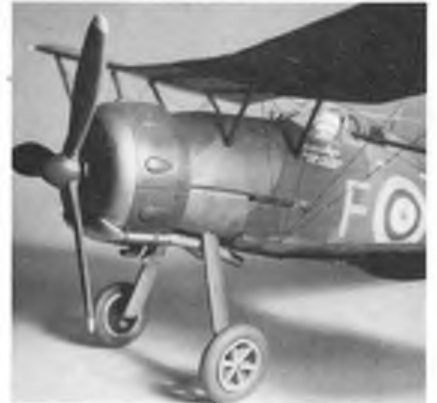
Left this underside view of the nose shows the CO filler protruding from the rear of the cowl Top details such as the pilot's name which can be seen on the side, and the compass within the cockpit, go a long way to achieving a realistic looking model Right this view of the wheels shows just what can be achieved with a balsa laminate construction.
