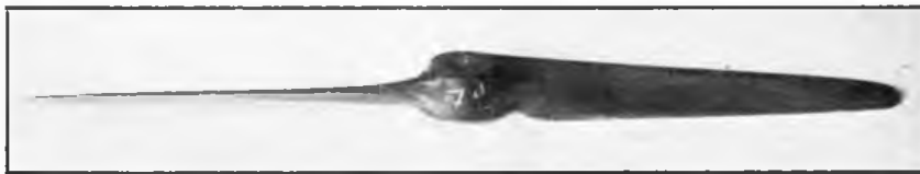
Above Larsson original with large hole for sleeved prop nut, and double diameter centre rod used to make mould
