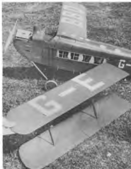
Above: John Coker's single-bay Spartan Arrow uses piano wire rigging. Note the neatness of the detailing. Right: transport and assembly are made easier if rigging wires terminate at the wing roots, allowing the wings to be removed as a cell. Note wire dowel wing fixing.
