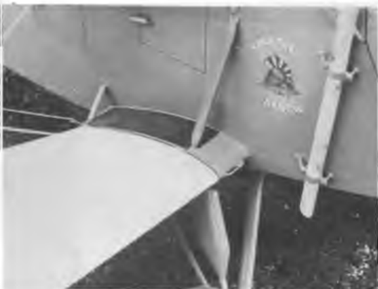
Above: John Coker's single-bay Spartan Arrow uses piano wire rigging. Note the neatness of the detailing. Right: transport and assembly are made easier if rigging wires terminate at the wing roots, allowing the wings to be removed as a cell. Note wire dowel wing fixing.
