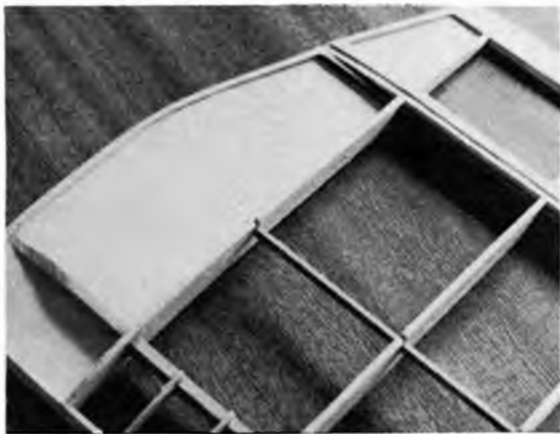
Wing tips are made in a similar manner to the tail surfaces, if you look closely at this picture you can see the small indentations caused by Bill Dennis' nails as he has formed the tip outline. Scale modellers take note not to bite your nails... even if your model is approaching terra firma from an unorthodox angle.
