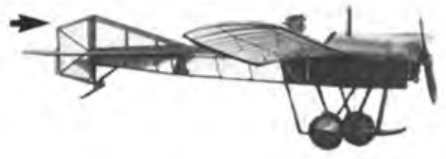
SUPERMARINE SPARROW by G. F. Eisegood 1/12th scale of 1920's light racing aircraft designed by R. J. Mitchell; 34 in. (864mm) span model features scale rib spacing and pendulum rudder/aileron controls. For 0.3-0.5 cc motors. FSP/1408 Price £1.65
