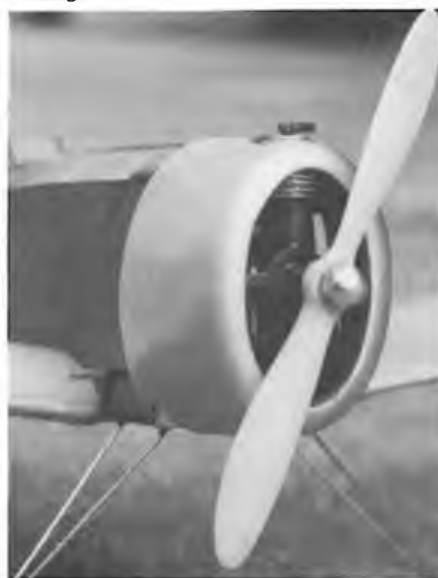
Above: detail showing local strengthening fore and aft of the wing mounting. Below: close up of front end showing simple but effective engine cowling.
