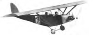
SUPERMARINE SPARROW by G. F. Eisegood 1/12th scale of 1920's light racing aircraft designed by R. J. Mitchell; 34 in. (864mm) span model features scale rib spacing and pendulum rudder/aileron controls. For 0.3-0.5 cc motors. FSP/1408 Price £1.65
