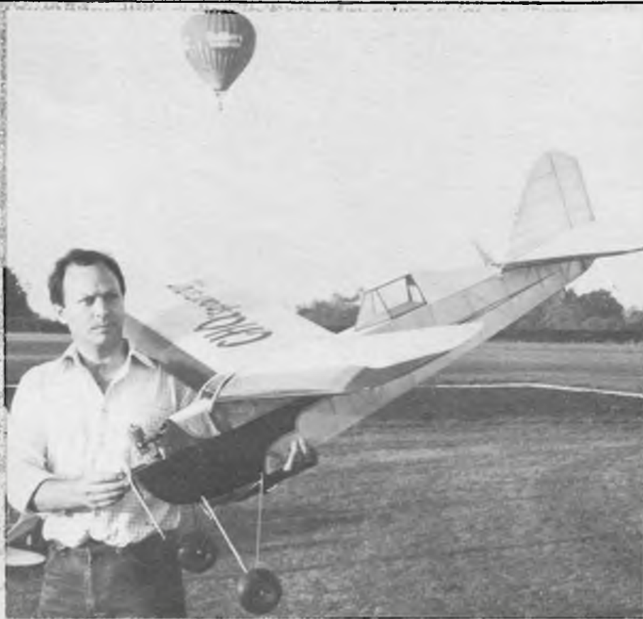
Above: MAP's Ron Moulton managed to include the Twilleys hot-air balloon in the picture when he shot Ian Potts with his 75in. span GHQ Sportster powered by an ETA5 diesel. This model designed by Julius Unrath was kitted by GHQ Models and was also described in July 1936 Model Airplane News. Right: P. A. Scorey with his DC Sabre 1.5cc diesel powered Air Trails Sportster at Old Warden during the South Midlands Meeting. The Sportster is a nice compact design by Ben Shereshaw originally described in September 1939 Air Trails, plans still available from MAP as PET/961 price £3.25 plus 50p postage. Below left: Marion has appeared in this column before, here she is again, this time with the float equipped Buccaneer Standard made by her father Peter Bull of Kilkenny, Eire (see text). Below right: G. W. W. Harris with one of his last streamlined Wakefields. This model is almost identical to his 1946 Wakefield Mk1 which was described in the January 1947 issue of Model Aircraft, plans of which are still available from MAP as MA 16 for £2.75 plus 50p postage.
