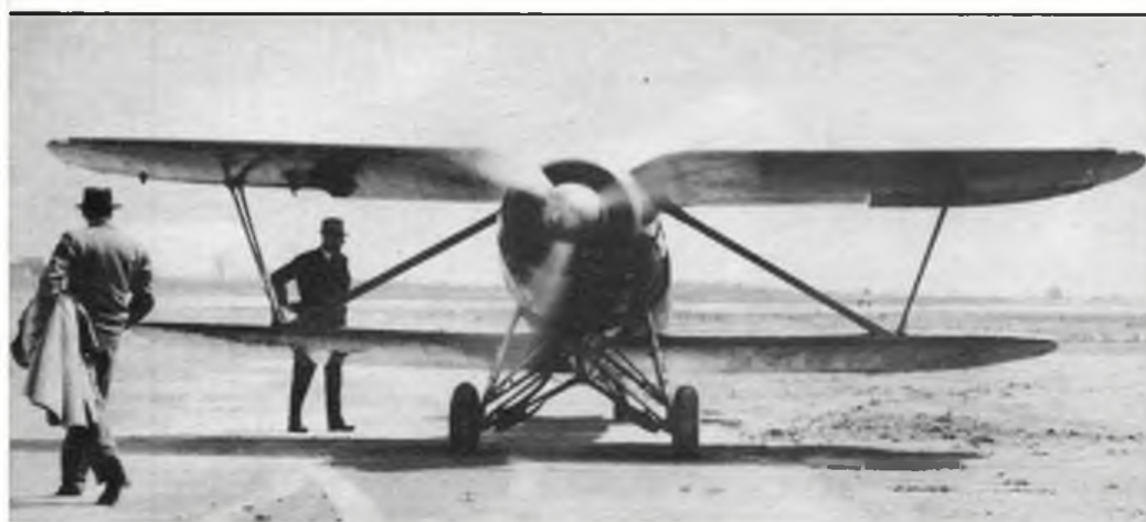
The final version with larger diameter spinner, hinges and operating horns visible beneath the ailerons and inset leading edge position lights replacing original external "fish eye" type at each upper wing tip.
