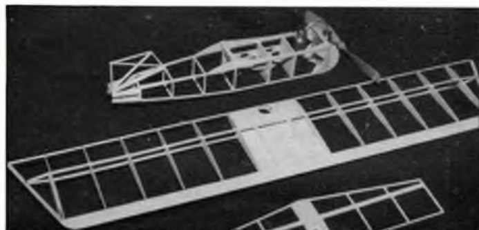
Component parts of 'Small Small Fry' before covering - care in wood selection and amount of glue used is important for good performance.
