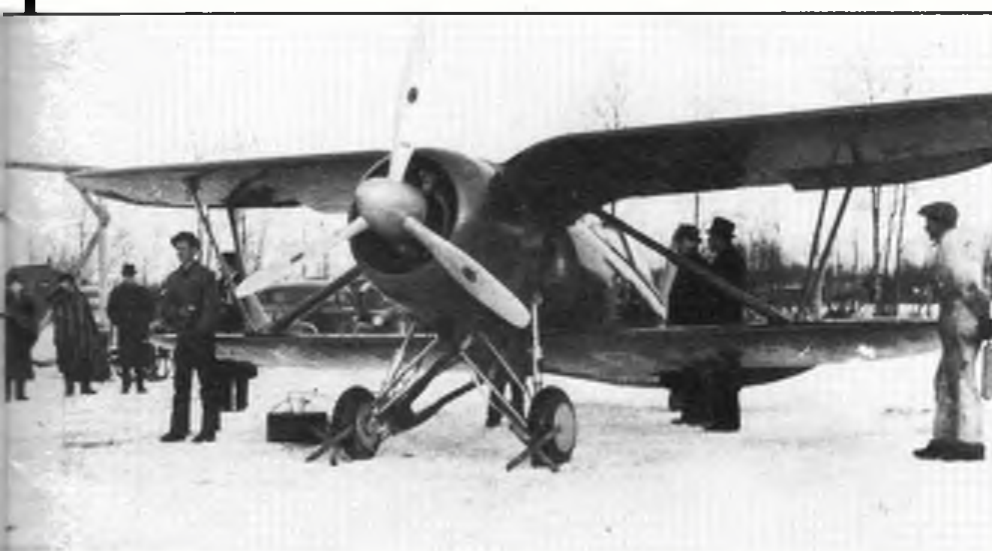
Taken during flight tests. The landing gear is now fitted with its regular radius rods and a spinner, slightly smaller than the final version, has been added, although there is little evidence of external aileron hinges or actuating horns.
