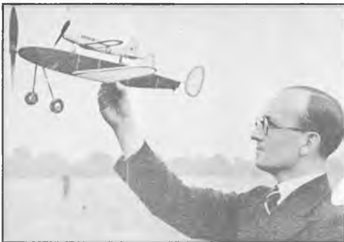
Above, MRK seen here with his first composite model which he flew on Wimbledon Common in May 1938. The 26 inches span carrier is the forerunner of a series of models that culminated in 'Kamlet' which was described in Aeromodeller 1941/42. The upper component is a Frog 'Raider' with its balsa mainplane suitably lightened.
