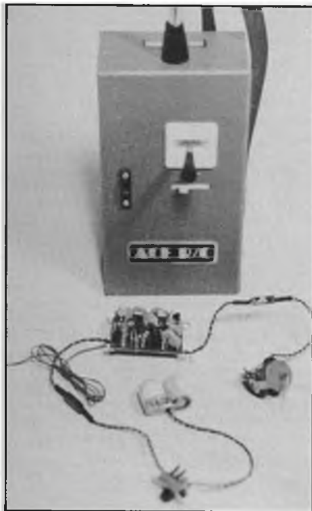
Above, so that you know what to look for... here is the total Ace system. Rudder wagging servo is seen to the right.
