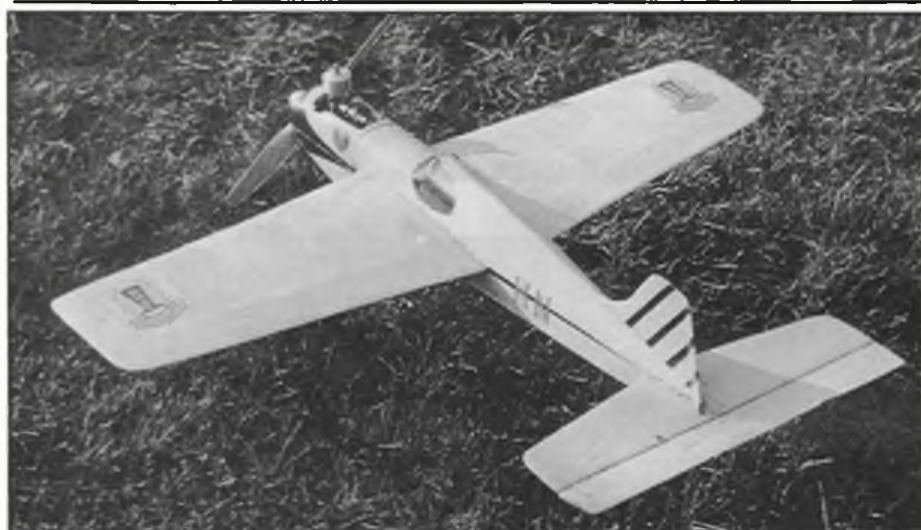
Top: A splendid period shot of Henry J. Nicholls' original Mercury Magnette. This stunt trainer from 1947 was powered by an ED Comp Special. Unfamiliar wing badges bear the legend 'SMAE Security'. Below: A nicely made Frog Vandiver, complete with manufacturer's insignia and Frog 180 diesel - the handiwork of Ray Gordon. How about a Frog prop instead of that Top Flite?
