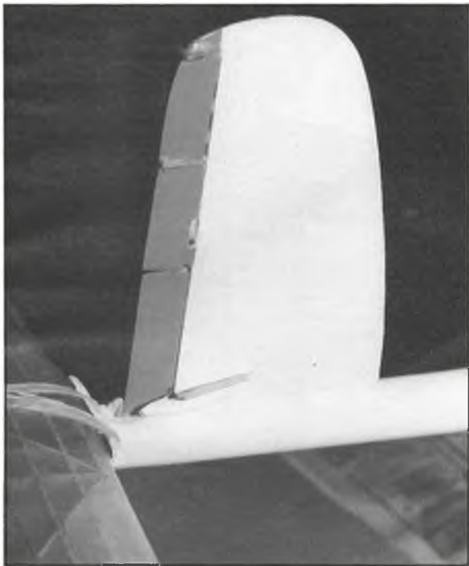
Opposite page: Tail and D/T line detail; the latter not yet hooked up. Autorudder in 'glide' position. Separated fixed sections are for fine trim. Below: Straightforward timer layout. All details on plan.
