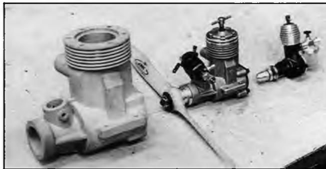
Bottom left: The Mace diesel. Centre: One of the last 'original' AM 15s, circa 1966. Note natural metal (not blue) head and brass in take insert. Bottom: A French Mills' - the Allouchery .7 from 1947. One for the replica makers?
