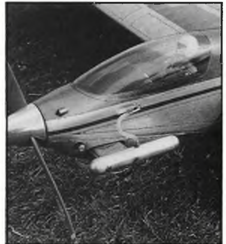
Neat cowl conceals a Merco 61 operating on silencer pressure, although motor operates well on suction too.
