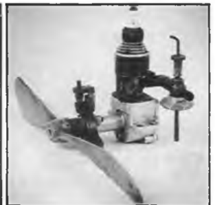
Bottom left: The Mace diesel. Centre: One of the last 'original' AM 15s, circa 1966. Note natural metal (not blue) head and brass in take insert. Bottom: A French Mills' - the Allouchery .7 from 1947. One for the replica makers?
