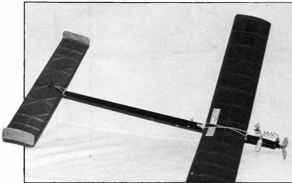
Vee-dihedralled 86B shown above. Triangular-section fuselage is rigid and light.
