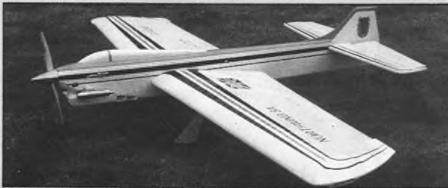
Neat cowl conceals a Merco 61 operating on silencer pressure, although motor operates well on suction too.
