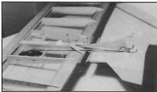
Detail of bolt-on tail experiment used on Fangle design (shown at foot of page). Note different wing sections of inboard and outboard panels. Swept-forward layout tried too!
