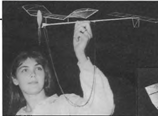
P15 class is for Indoor designs of 15in span. 'Standard' category at Wigan was for Erik Knudsen's version (drawing below) with tissue, condenser paper or clingfilm covering.
