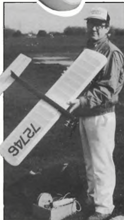
Above: Tom Dixon's sleek, enlarged Thunderbird MkII is 62in span, has 744sq in area and weighs 64oz for its Merco 49.
