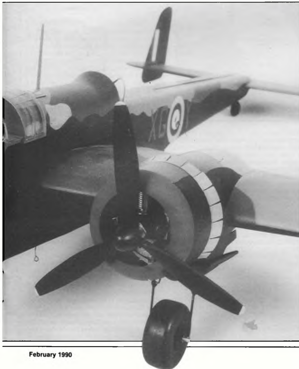
Retract-undercarriage linkage appears complex but is straightforward in action. Refer to diagrams overleaf.
