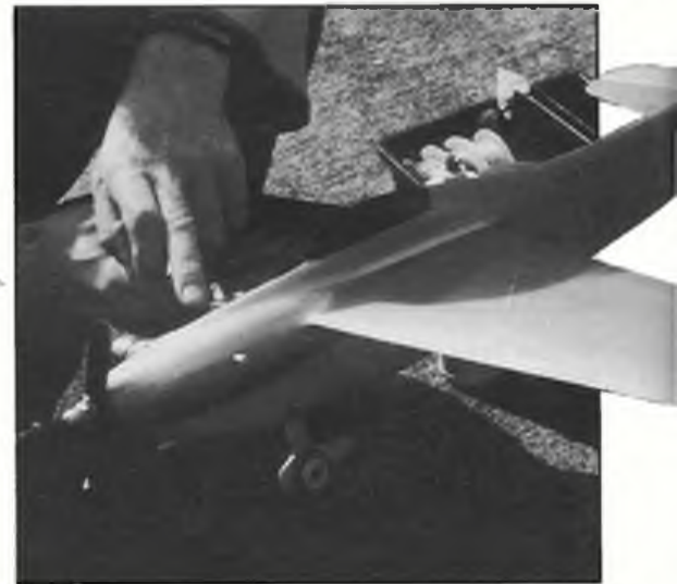
Neat Goodyear racer seen at the Nats - undercarriage leg pivot reveals use of wobbly wheel
