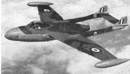
■ X 787 was the third production Venom NF 3 for the R.A.F., seen in maker's colours prior to delivery. In service, the radome is usually matt black, not grey as here. Note camouflage pattern and clean jet orifice which immediately distinguishes the land based Venom from its carrier-borne counterpart. (D.H. Photo.)
