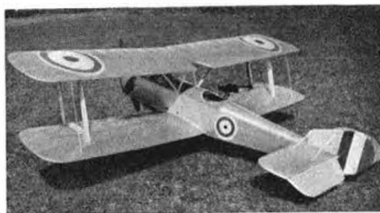
All sheer with blue/grey decking signifies R.N.A.S. markings for Brian Sichi's prototype Sopwith 1 \frac{1}{2} Strutter fitted with a Frog 500. Note the generous tail surfaces and ideal proportions of this full stunt model.
