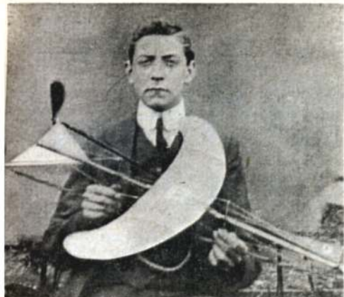
Record holder with an 89 sec. flight in 1912, young Alex Houlberg shows his twin pusher with T-frame and sweptback wings
