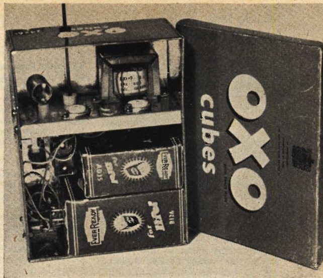
How it fits in the OXO tin—batteries need foam packing and in this view, valves and Xtal are detached. Meter socket is at lower left side. Tuning hole half way up same side, switches on front face
