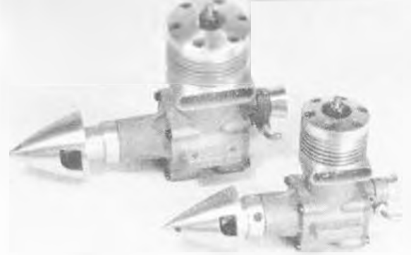
Schuco Hegi Frechdax above now nears completion and looks a very nice robust model. Note the Spinaflo silencer fitted to Enya .09 power plant.
