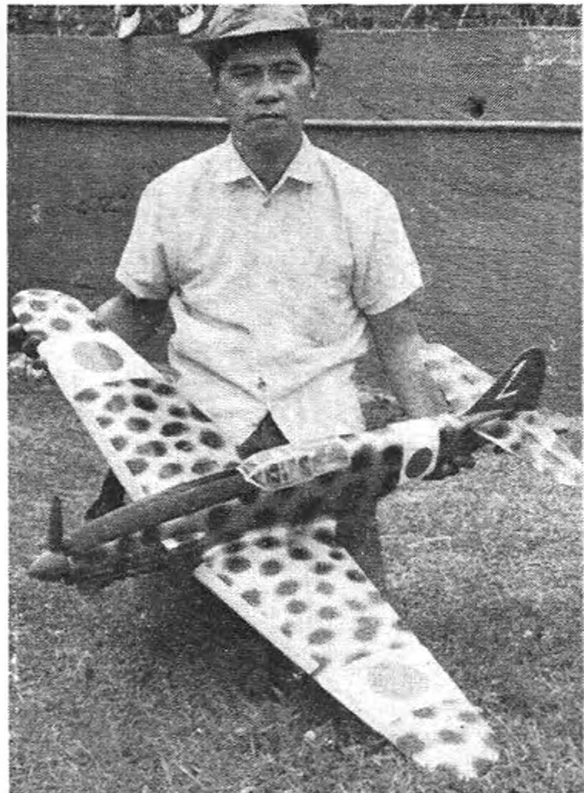
Above: Japanese C/L scale Tony is by Thori. This model has third line control to operate throttle on O.S. Max H 40 R/C. Below: Sleek speed model by Nakamura of Japan which is powered by O.S. Max H60R, set up the new Japanese speed record for 10 cc. models at the "All Japan Contest" with 165 m.p.h.
