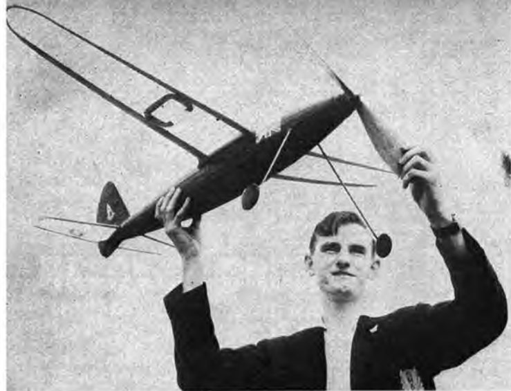
The beautifully streamlined Wakefields (above) by R. N. Bullock, with their clean, plug-in shoulder wings probably date from before 1937, but it was with one of these that he secured second place in the 1937 Wakefield contest. He used the same model in '38 and similar layouts were used by Copland (seen at left) and Chasteneuf. Highly refined, they were 'caviar to the multitude'.
