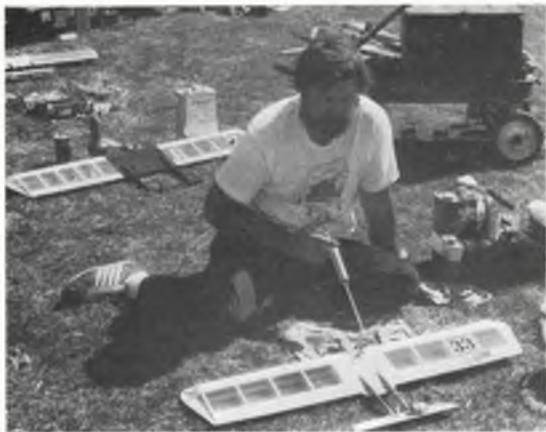
Seen at the WAM contests. Left: 'The Master' Edmond Bridant uses extra long syringe to re-fill the pacifier tank on his Fast Combat model. Above is Ira Keeler's model for the same event - note plastic clunk-tank rubber banded to leading edge.
