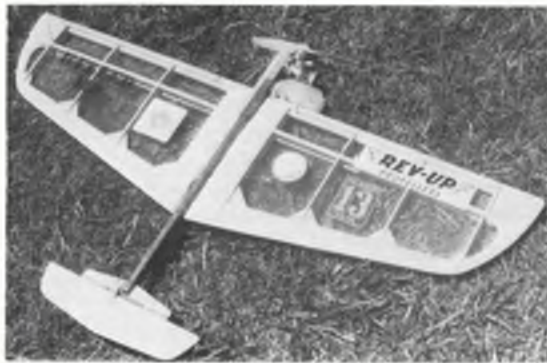
Seen at the WAM contests. Left: 'The Master' Edmond Bridant uses extra long syringe to re-fill the pacifier tank on his Fast Combat model. Above is Ira Keeler's model for the same event - note plastic clunk-tank rubber banded to leading edge.
