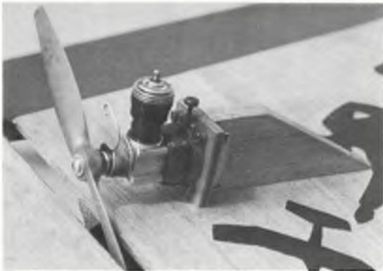
Picture up shows the engine installation with the prop running in a slot in the wing and 'fuselage'. At right is the completed machine—leaves ample scope for decorating with your own pet colour scheme, or design a suitable traffic sign! However, remember to go easy with the amount of paint used – a heavy airplane is a fast-flying one.
