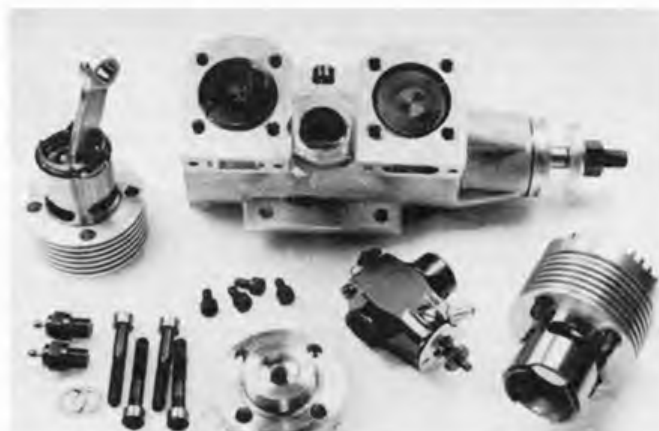
B&C 61 uses lapped cast-iron pistons running in steel liners. Carburettor is much-modified Perry
