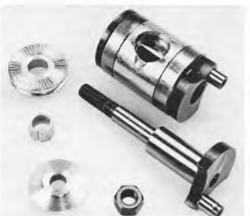
B&C 61's unusual shaft setup features permanently assembled centre unit comprising crankcase divider, twin ball bearings and dual rotary valve ports in centre journal
