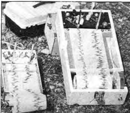
Victorious Lothar Doring holds high the famous Wakefield Trophy. Below: Doring's two twin chart recorders plot temperature and wind speed for comparison, pens moved by R/C servo motors. Below right: 3-D turbulator cut into leading edge of solid balsa wing on winning Wakefield (see p.89 Feb. '81 issue for full details).
