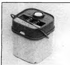
Right: Mabuchi A1 charger unit, holds two U2 batteries which give a 1 amp charge by depressing the button on top for five minutes.
