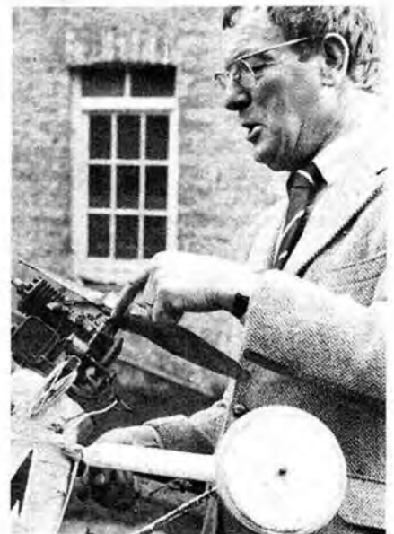
Colonel Bowden's 1932 'Kanga.' The engine is a 28cc Wall modified by Edgar Westbury. Right: Alex Imria is discussing various points about the engine with the Colonel. Note the rubber bands holding the engine mount in place and the large wheels, probably obtained from a local ironmonger.
