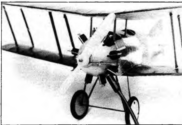
Fine engine detail of the author's Nieuport Nighthawk which illustrates the fine engine detail made possible with electric power. Note the charging lead inserted at the bottom of the engine cowl.
