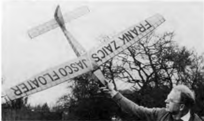
Right: Cliff Billington with his Korda Wakefield. This popular 44in span model was kitted in this country by Skylada and sold for 17/6d (87p) in 1947. Below: no doubt about the identity of this glider that the SAM 35 'sparkplug' is holding. Designed for fast construction and low cost, this 6ft span model was described in the book 'Model Glider Design 1944'.
