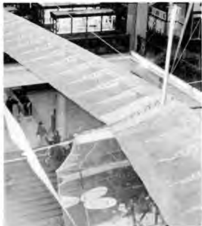
Paul MacCready's 'Gossamer Albatross' man-powered aircraft, which flew across the English Channel in June 1979 to win the Henry Kramer prize of £100,000. Now on view at the London Science Museum
