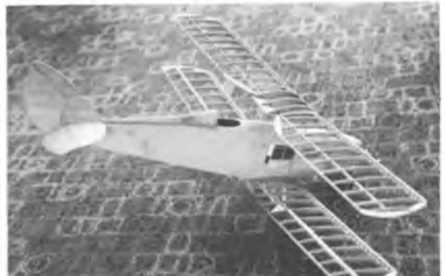
Above: Air Travel NZ Ltd. logo is painted in red on a silver background. Right: completed structure of the model, note bulge in cabin door.
