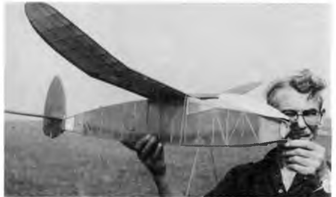
Right: Cliff Billington with his Korda Wakefield. This popular 44in span model was kitted in this country by Skylada and sold for 17/6d (87p) in 1947. Below: no doubt about the identity of this glider that the SAM 35 'sparkplug' is holding. Designed for fast construction and low cost, this 6ft span model was described in the book 'Model Glider Design 1944'.
