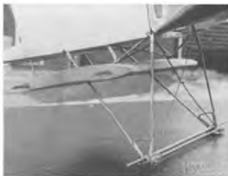
Left: instead of bolting your engine directly to the bearers, mount it indirectly via a dural plate which allows easy thrustline adjustments. Below: on a Bristol 'Fighter' it is not possible to have the u/c legs swing back. Michael Smith has made a strong structure and relied on axle springing. Right: the tailskid on the Bristol is also built to last!
