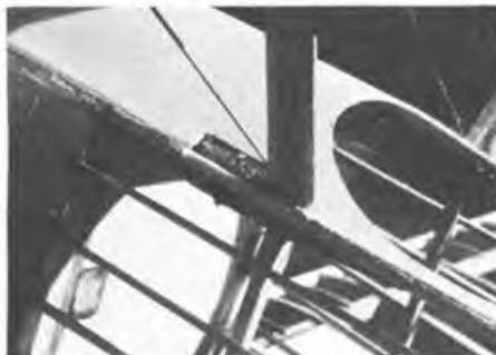
Above: here the rear cabane struts fall in the cockpit area, so they are mounted on the locally reinforced longerons. Below left: the 'Arrow' ready for covering. The shapes at the aileron tips are more complex than usual. Note tail surfaces are built on traditional lines. Below right: stringers on the 'Pup' are shaped to a knife edge. The supplementary \frac{1}{8} in. ply full depth formers can be seen, also the strips glued to the longerons to support the covering.
