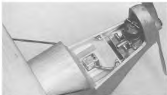
Left: instead of bolting your engine directly to the bearers, mount it indirectly via a dural plate which allows easy thrustline adjustments. Below: on a Bristol 'Fighter' it is not possible to have the u/c legs swing back. Michael Smith has made a strong structure and relied on axle springing. Right: the tailskid on the Bristol is also built to last!
