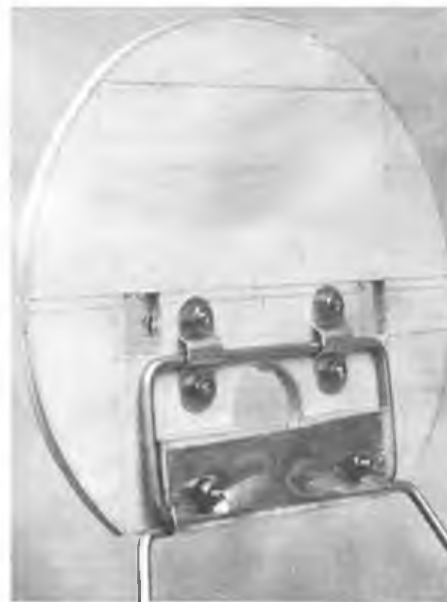
Above: torsion bar u/c mounted on the Sopwith 'Pup's' front bulkhead before assembly. Below left: the first step in assembling the 'Pup' fuselage. Note gussets reinforcing the longerons where they have to be cracked. Below right: the firewall butts onto the front fuselage and the bearers glued to the sheet sides. Use Araldite for these joints.
