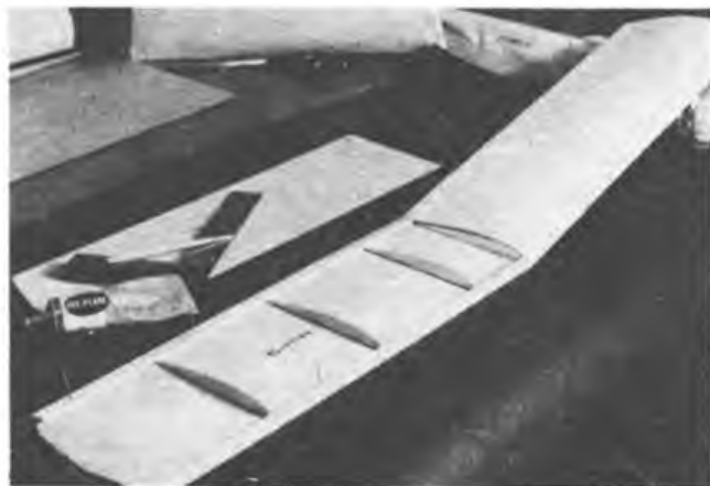
Left: showing the simple construction of Pulstar's wings, being all sheet they provide a durable, fairly crashproof structure but be sure to use light sheet. Below and below left: wing construction detail, note the use of adhesive tape to hold wing sheeting whilst glue sets. Far below: major construction finished, check alignment of wings and tail before continuing.
