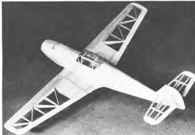
Cedric de la Nougerede's 1/10 'Tiger Moth' demonstrates its strongly built cabane structure. In this case, Cedric has soldered the wing dowels directly to the cabane. Right: Cedric's Me109 is built on the same lines as his APS 'Mustang'. Fuselage is a horizontal crutch structure sheathed over formers.
