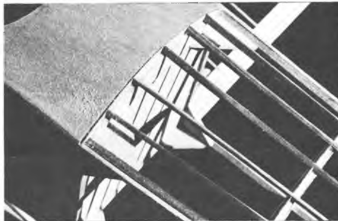
Above: here the rear cabane struts fall in the cockpit area, so they are mounted on the locally reinforced longerons. Below left: the 'Arrow' ready for covering. The shapes at the aileron tips are more complex than usual. Note tail surfaces are built on traditional lines. Below right: stringers on the 'Pup' are shaped to a knife edge. The supplementary \frac{1}{8} in. ply full depth formers can be seen, also the strips glued to the longerons to support the covering.
