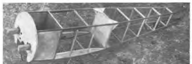
Above: torsion bar u/c mounted on the Sopwith 'Pup's' front bulkhead before assembly. Below left: the first step in assembling the 'Pup' fuselage. Note gussets reinforcing the longerons where they have to be cracked. Below right: the firewall butts onto the front fuselage and the bearers glued to the sheet sides. Use Araldite for these joints.
