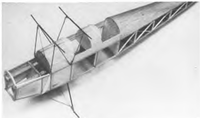
Cedric de la Nougerede's 1/10 'Tiger Moth' demonstrates its strongly built cabane structure. In this case, Cedric has soldered the wing dowels directly to the cabane. Right: Cedric's Me109 is built on the same lines as his APS 'Mustang'. Fuselage is a horizontal crutch structure sheathed over formers.
