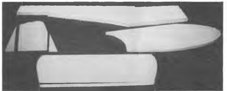
The following pictures will help the novice, when building Pulstar. Left: layout of major components, marked out ready for cutting. Below far left: fuselage is from 1/2 in. sheet, easier to cut using a fretsaw than with a knife. Below left: sanding fuselage parts roughly to shape. Below: components ready for gluing.
