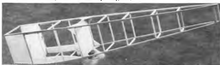
Above: torsion bar u/c mounted on the Sopwith 'Pup's' front bulkhead before assembly. Below left: the first step in assembling the 'Pup' fuselage. Note gussets reinforcing the longerons where they have to be cracked. Below right: the firewall butts onto the front fuselage and the bearers glued to the sheet sides. Use Araldite for these joints.
