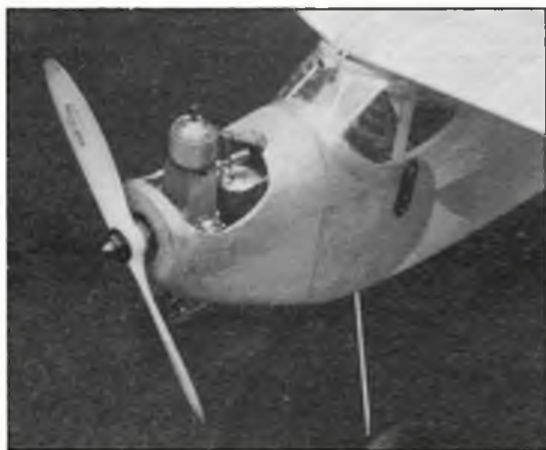
The 48in. span 'Hepcat', shown here with Replica Mills Mk I 1.3 cc engine, fine for free flight, but not so ideal with the added weight of R/C gear.
