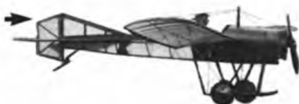
SUPERMARINE SPARROW by G. F. Elsegood . 1/12th scale of 1920's light racing aircraft designed by R. J. Mitchell; 34 in. (864mm) span model features scale rib spacing and pendulum rudder/aileron controls. For 0.3-0.5 cc motors. FSP/1406 Price £1.80
