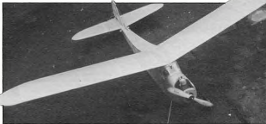
Above, the attractive lines of the 'Hepcat' have led to thousands being built over the years. Jim's version has R/C assist. Below, the original Mills Mk I found the going a little difficult with 2 1/4 lbs. to pull around, so a modern PAW 1.49 took over. The K.K. tank is epoxied to a shelf resting on the bearers.
