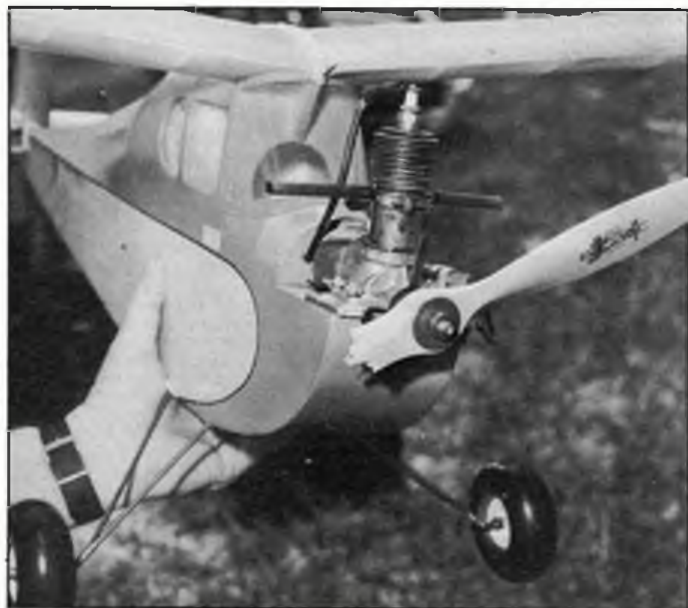
The bane of freeflighters. Stouffer photo of Joe Beton's Brown B Ignition powered 'Buzzard Bombshell', taken at Bong in June 1984 showing the curse of freeflighters - the broken wooden propeller blade. A candidate for the treatment outlined in the text!
