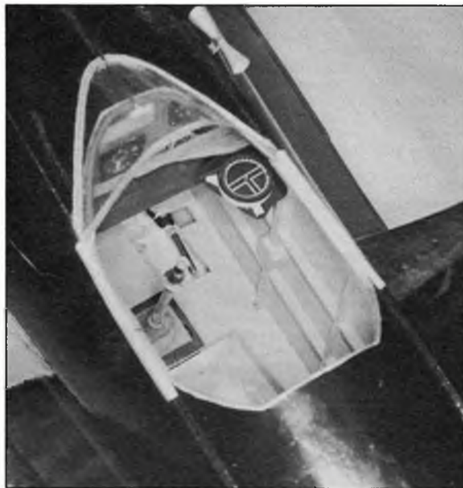
Compass and control column detail on the Fox Moth; note gaiter on the latter and 'weathered' effect on front edge of seat.
