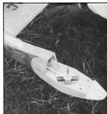
Heading, Madeleine Bodmer with her favourite F1E magnet flier 'Illuc'. Centre, a spot of trimming on the local flying field with the latest model, 'Radulina'. Madeleine has her sights set on a place in the Swiss National Team. . . Above, magnet bay on 'Illuc'; pivotted bar magnet has pushrod connection to rudder and contributes to noseweight.
