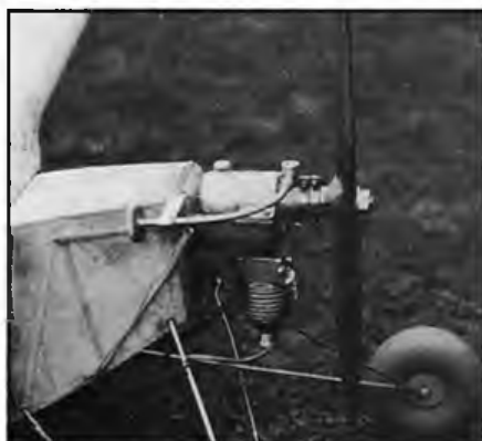
Above photos: A.E. Brooks' original 58in. Comet III which was fitted with a 2.5cc Baby Spitfire petrol engine. Despite its name this was really a reduced-size Brooks' Skyrocket. Left: Close-up of the engine installation. Note the flexible needle valve extension, meant to keep fingers away from the propeller. See also this month's opening paragraph.
