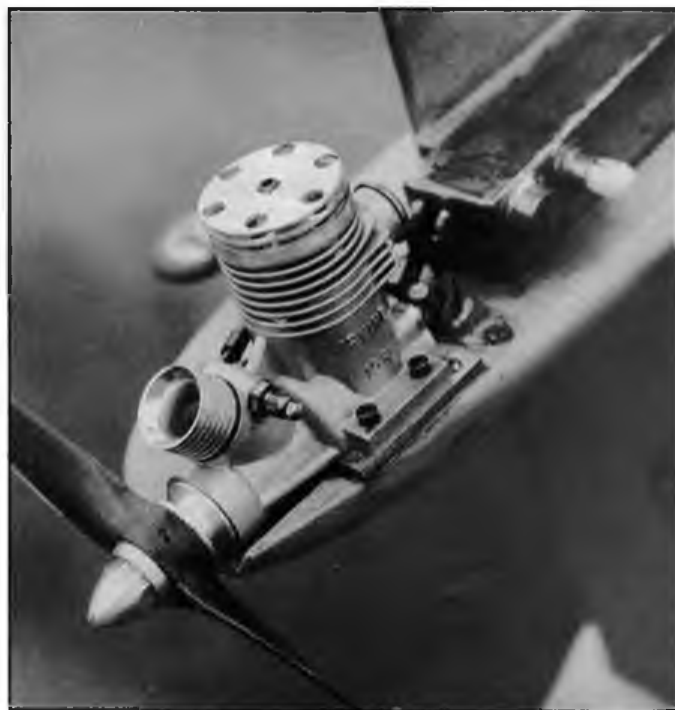
Above: Peter Chinn returns on p.136 to review the Irvine .15R glow. This is Ed Needham's 'dieselised' version which was flown to such good effect at the 88 Nats by Dave Clarkson, creating a new Open Goodyear Record in the process. Below: A wry look at the therapeutic value of aeromodelling in Terry Rose's view...
