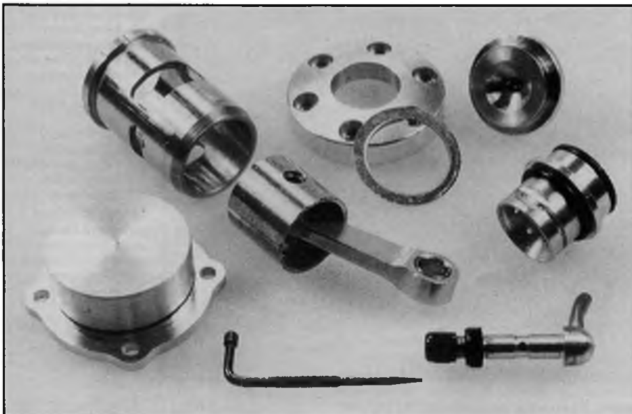
Irvine 15R features thick-walled chrome-bore brass cylinder liner with general, well-shaped parts. Note also the two-part head.
