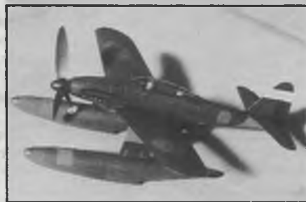
Antonin Atery's Aichi Seiron for Peanut Scale features foam construction. Brave subject with those drag-inducing floats.
