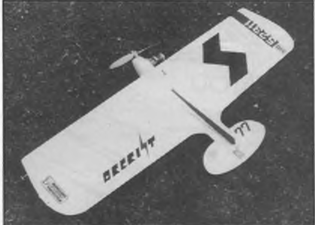
Frank Smart's own Orcrist is covered in Solartex. Weight 14.1/2oz - very competitive for a 1970 design. Left: Engine pod is pre-covered with Solartex.
