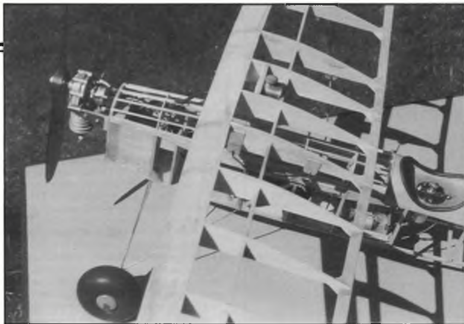
A close-up showing fuel tank in wing centre section, aluminium tabs for wire cabane strut ends and Austin timer in cockpit.
