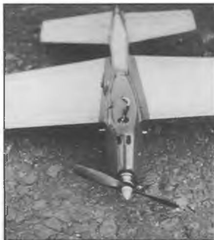
Underside of nose. Visible are the 'puffer' head air inlets, and bent wire plug chip.
