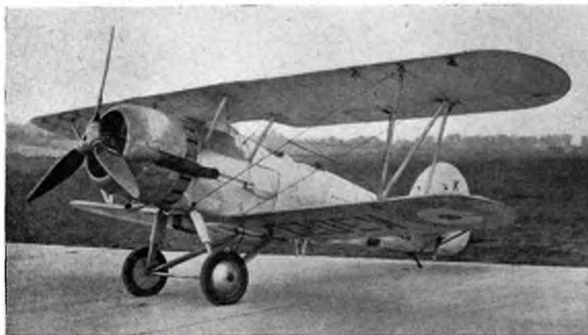
Above is shown a Hawker "Hart" fitted with a Bristol "Perseus" sleeve-valve aero engine, and "Rotol" airscrew for flight testing. On the right is shown one of the American Northrop all-metal monoplanes, fitted with Bristol "Hercules" sleeve-valve engine.
