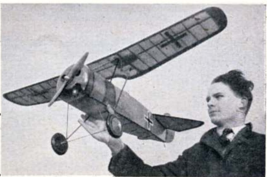
Top photo: An outsize in free-flight scale is the massive 16 lb. Tiger Moth by A. Manley of Dover. The 7 ft. Eros looks small by comparison! Right: V. Mills scaled up his Keilkraft kit to 48" span for his Elfin 2-49 Fokker D.VIII. The axle 'wing' was removed after being damaged.
