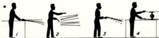
1. A BUNDLE OF STRIPS SUPPORTED OVER EDGE OF TABLE, THE LIGHTEST WEAKEST STRIPS BEND FIRST. CHOOSE FOUR STRIPS OF THOSE REMAINING STRAIGHT. 2. A BUNDLE OF STRIPS DROPPED, THE HEAVIEST STRIPS REACH THE FLOOR FIRST. 3. WHIP FOUR OR MORE STRIPS TOGETHER. MATCHED STRIPS WHIP THE SAME AMOUNT. 4. FINALLY, CHECK THE WEIGHT OF STRIPS. FIG. 4.
