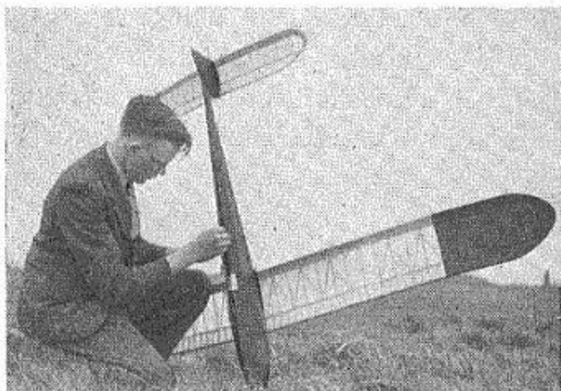
Roy Grasmeyer of West Essex sets the D/T on his glider before a contest flight. In this case, the dethermaliser fuse is fitted amidships, like that on the "Arrow", which has a tip-down tail, on page 217.
