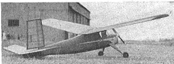
Neat "Valkyrie", 6 ft. 0 in. cabin job for the E.D. 346 diesel is by Jim Robbie of the Mercury M.A.C., Musselburgh, Midlothian. Background is the Club's Macmerry airfield, used by permission of the Edinburgh Flying Club.
