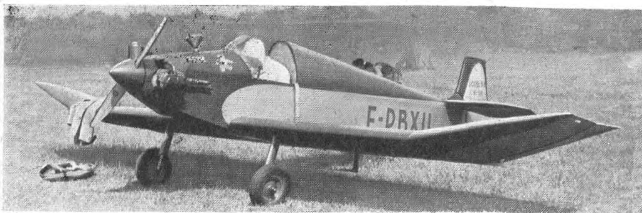
Left, is another visiting Bébé, also the work of its pilot, Andre Rubichon, seen here in the cockpit. Both these machines have curved metal spinners instead of a standard conical plywood type.
