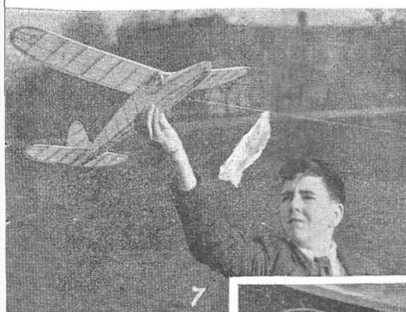
6. Wire ring and tuft of lightweight silk on the end of the white cotton towline. 7. How the assistant should hold the model for towing up. Note the marked way in which the nose is pointed upwards. 8. All ready for the great moment, with the breeze blowing straight down the line from the launcher to his assistant. 9. How NOT to tow up a glider. Running backwards can very often result in the launcher ending up flat on his back! 10. As you move forward, always keep looking over your shoulder like this, so as to
