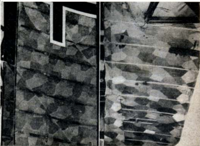
Below left: The Halberstadt C.V. hanging in the Musee de l'Armee in Brussels has its fabric covering at an angle of approximately 45 deg. and uses a mixture of both four and five colour patterns on various parts, see text. At right is H. D. Hastings' picture of the Albatros D.Va. in the Canberra War Museum showing how an additional strip is used at the trailing edge to make up full width
