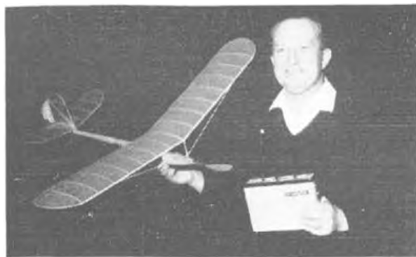
First to fly radio underground? Fred Militky, designer for Graupner in Germany and his ultra lightweight model after a successful flight last year. Model is 36 in. wing span and weighs 2.46 oz. ready to fly using specially prepared Grundig radio. Micromax T 03/15 electric motor which is the heaviest single component, drives a Silentius type propeller. Flight is at slow speed enabling simple magnetic rudder control to be fairly non-sensitive.
