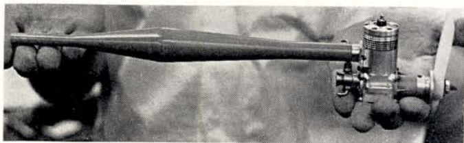
Bill holds latest experimental K & B 15 above with tuned length exhaust pipe. Increases 24,000 to 26,000 R.P.M. and reduces noise!
