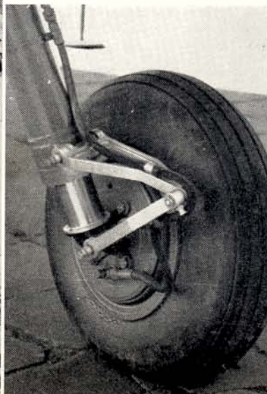
Details in the Wilga 2 close up of show earlier under-carriage which is easier to reproduce.
